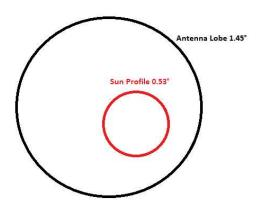
We know that the angle subtended by the Sun's disk holds **0.53°** which correspond to a surface of **0.22** degrees<sup>2</sup>, the beam of our parabolic antenna is worth instead **1.45°** which correspond to **2 gradi<sup>2</sup>**.
