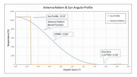
Since the radiation pattern of solar radiation is much narrower than the antenna pattern, the convolution of the two functions will be very similar to the somewhat enlarged antenna pattern. However, we have not done the calculation but the graph obtained from the registration of the transit, which we report below in "angular" terms instead of time, has the expected trend.
