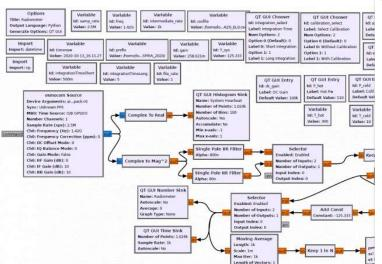
The **osmocomm source** block is the interface with the Airspy R2 SDR hardware the bias-T option so in the argument string we have put "airspy = 0, bias = 0, parameter can be set to 2.5 MHz or 10 MHz, these values correspond to a use the first case and 10 MHz in the second. The Frequency parameter is set at 1
