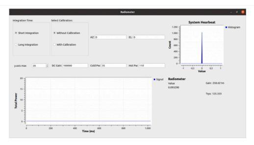
**Abstract**: In this post we continue the description of our diy microwave radio telescope. In the first part: A simple 11.2 GHz RadioTelescope (HW Part) we have described the hardware part of the instrument, including the parabolic reflector antenna, the LNB block and the receiver. Now we take care of the software that does the measurement of the signal strength and its integration over time.
