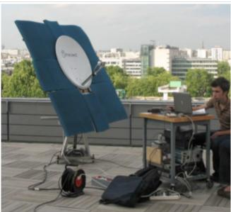
Stein and Förster use a cylindrical collar (about 1.5 m length) of aluminum foil put around the rim of the reflector (diameter 1m). The foil is wrapped around a cylinder formed with chicken wire fence material (with mesh size 13 mm)
