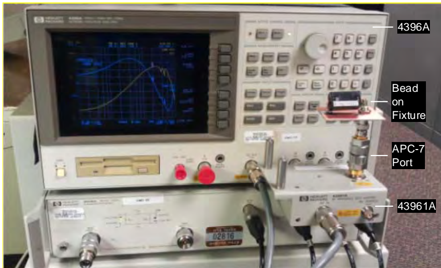
Lower: The H-P 4396A VNA with 43961A Impedance Test Kit shown with the Short test fixture and a clamshell bead. The 43961A is first calibrated using HP SOL calibrated references directly at the APC-7 port. Then an APC-7 to BNC adapter is connected at the port and is compensated with each of the custom Short, Open, Load fixtures.
