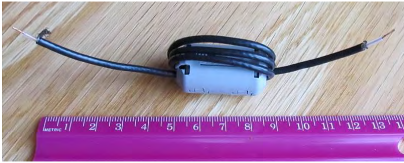
Figure 4 ~ Clamshell ferrite bead with four windings of RG-174/U coaxial cable. The bead is a very common TDK p/n ZCAT-2035-0930 and has a 9 mm inside diameter.
