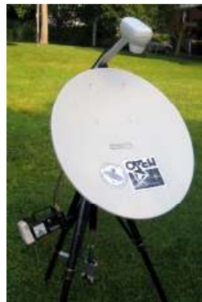
An IBT showing the LNB on top for easier aiming, the DSS dish, the Channel Master (bottom left) with amplified speaker, and the battery pack below.
