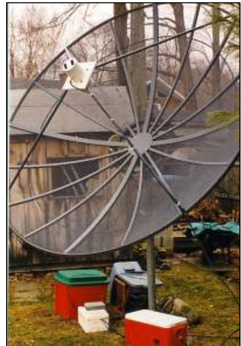
My 1420 MHz Total Power Telescope – 10' dish with horn leading to temperature controlled LNA, IF Amp, detector (in cooler), then leading to voltage amp (foam box), then to A/D device and computer (in plastic bin). Power supplies are on wooden stand.
