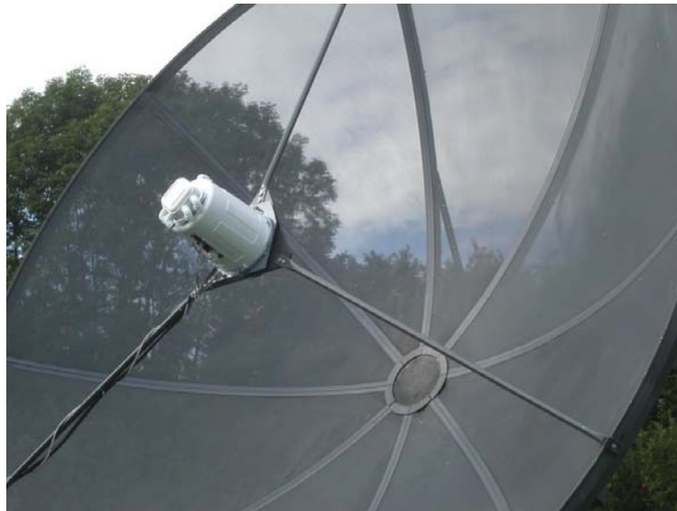
Figure 1 3m diameter dish with integrated feed / LNA
